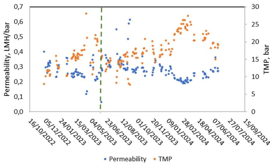
Figure 7. CS1: Reverse osmosis permeability and transmembrane pressure. Green dotted line shows CIP cleaning.
