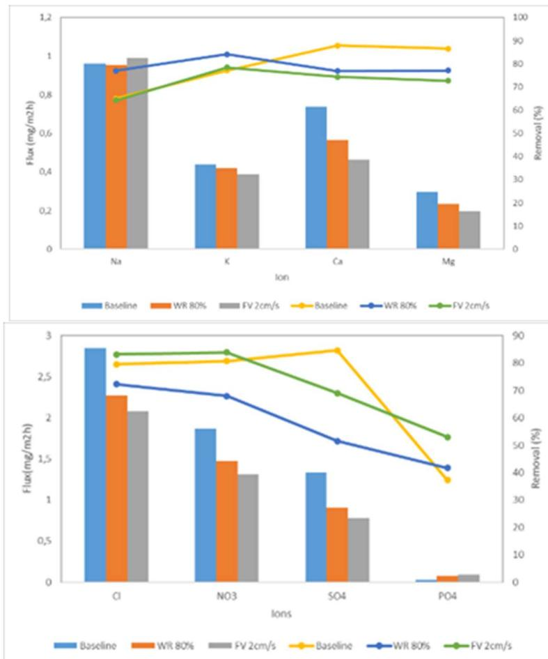
Figure 15. CS2: Effect of variable ED parameters - flow velocity (1 and 2 cm/s) and water recovery (50 and 80%) on ion flux and removal of the reclaimed water.
