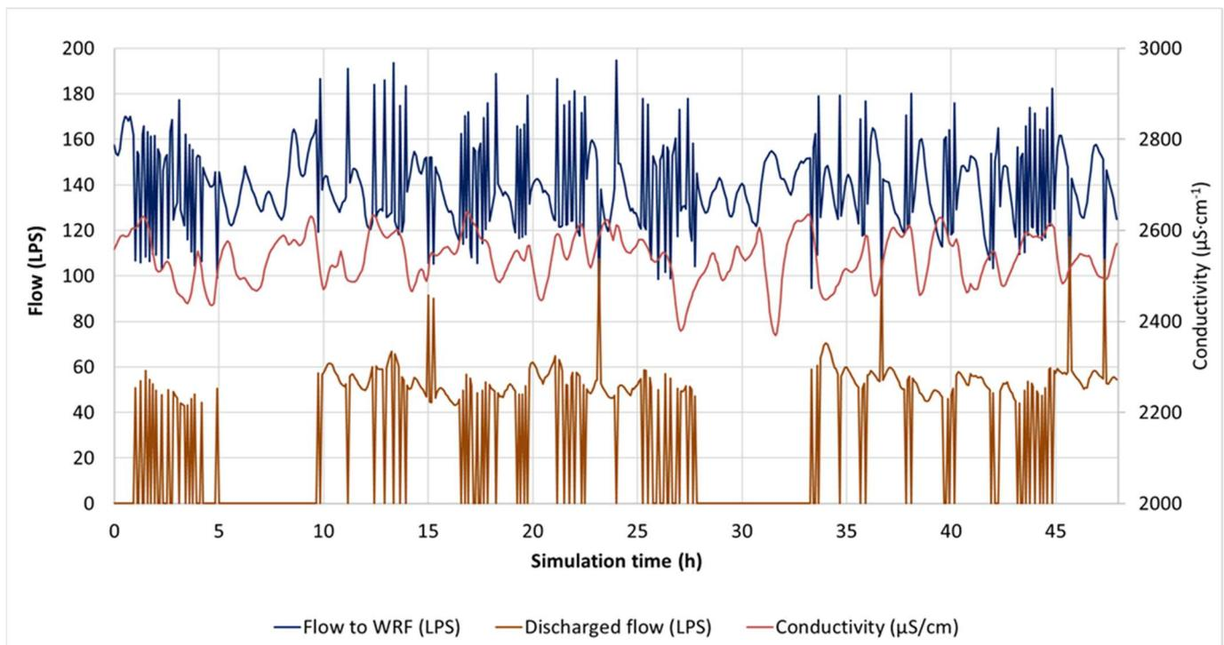
Figure 27. CS3: Distribution of the water flows carried out by the smart equalization system.
