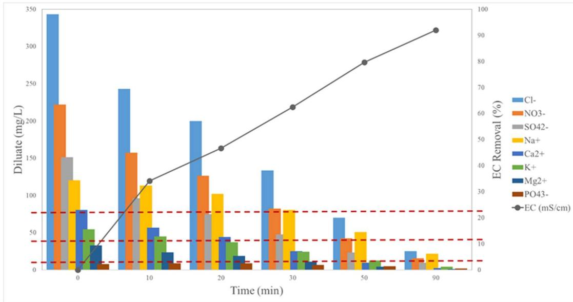
Figure 13. CS2: EC removal and ionic water quality of the irrigation water for reuse (diluate) with the baseline conditions for reaching the target conductivities (EC in the range of 1, 0.5 and <0.2 mS/cm, represented by the red dotted lines).
