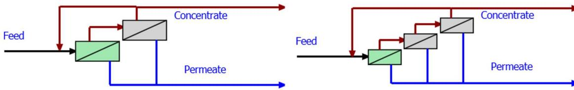
Figure 63. CS9: Design of full-size RO, left: 2-stage RO; right: 3-stage RO.
