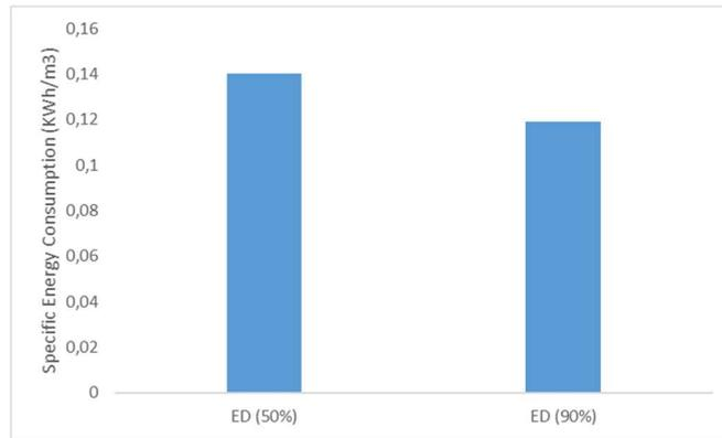
Figure 16. CS2: Specific energy consumption (kWh/m<sup>3</sup>) for 60% and 90% water recovery.
