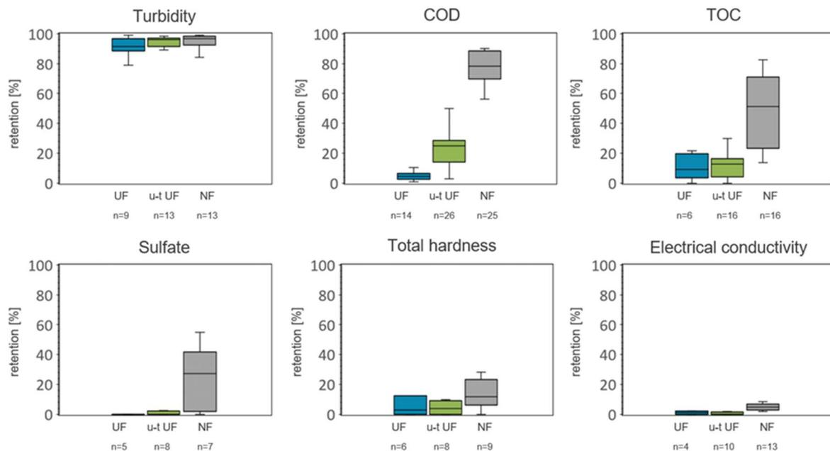
Figure 61. CS9: Performance of UF, u-t UF and NF: removal of selected parameters with number of samples.
