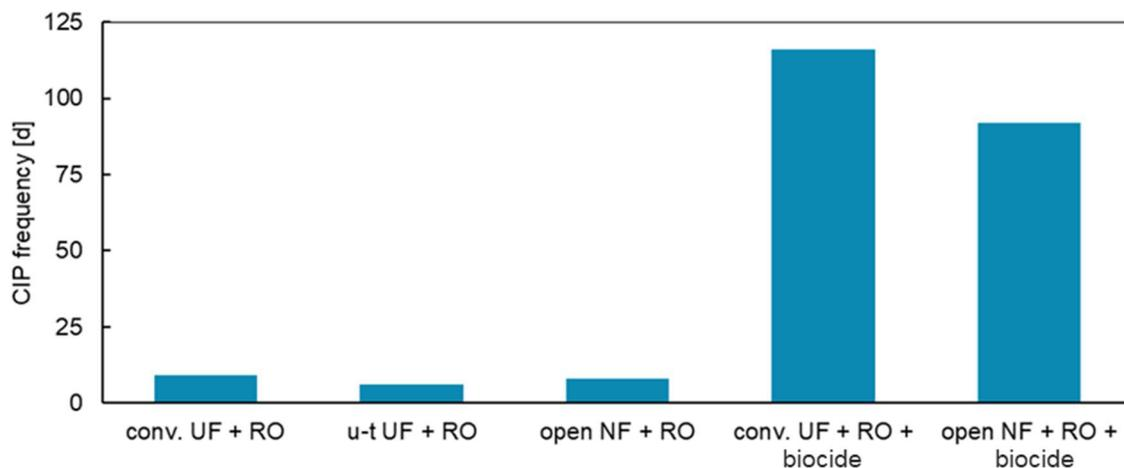
Figure 64. CS9: CIP frequency of RO calculated using the hydraulic pressure difference.
