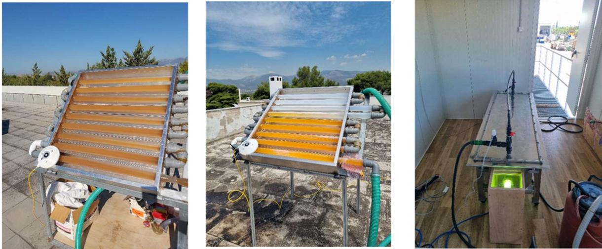
Figure 41. CS4: Photocatalytic reactor.
