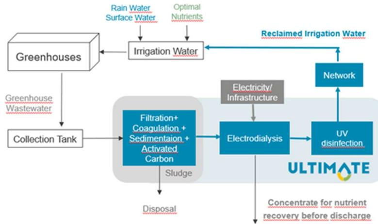
Figure 12. CS2: Treatment scheme and proposed Ultimate technology solution for the wastewater treatment plant at De Vlot.
