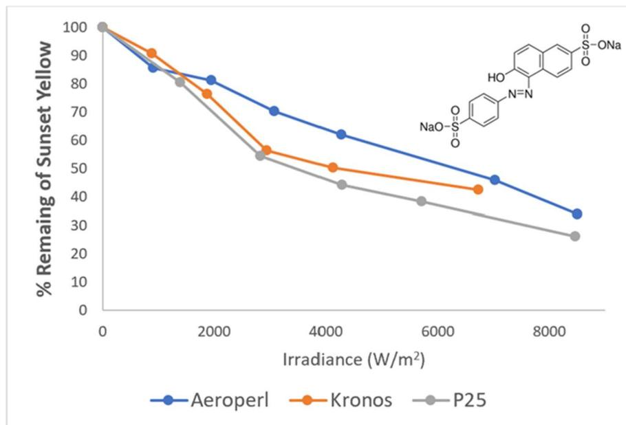
Figure 46. CS4: Degradation of a model organic compound using the CPC solar reactor.
