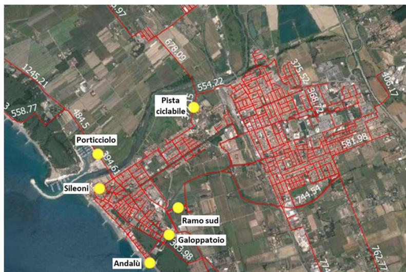
Figure 31. CS3: Flow meters already installed in the municipality of Cecina (of which 3 are reliable: Porticciolo, Sileoni and Galoppatoio).
