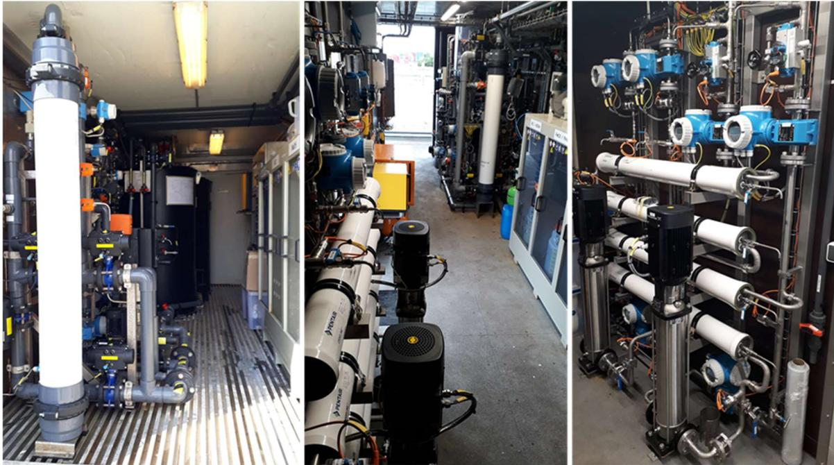
Figure 59. CS9: View inside the pilot plant: left: pilot container A (UF/NF); middle: pilot container B (UF/NF); right: pilot container B (RO).
