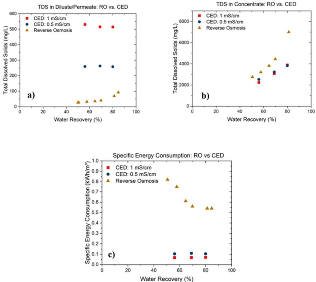
Figure 19. CS2: Comparative evaluation of capacitive electrodesalination (CED) and reverse osmosis (RO) Technologies for a) ion removal performance, b) concentrate generated (TDS), and c) estimated SEC.
