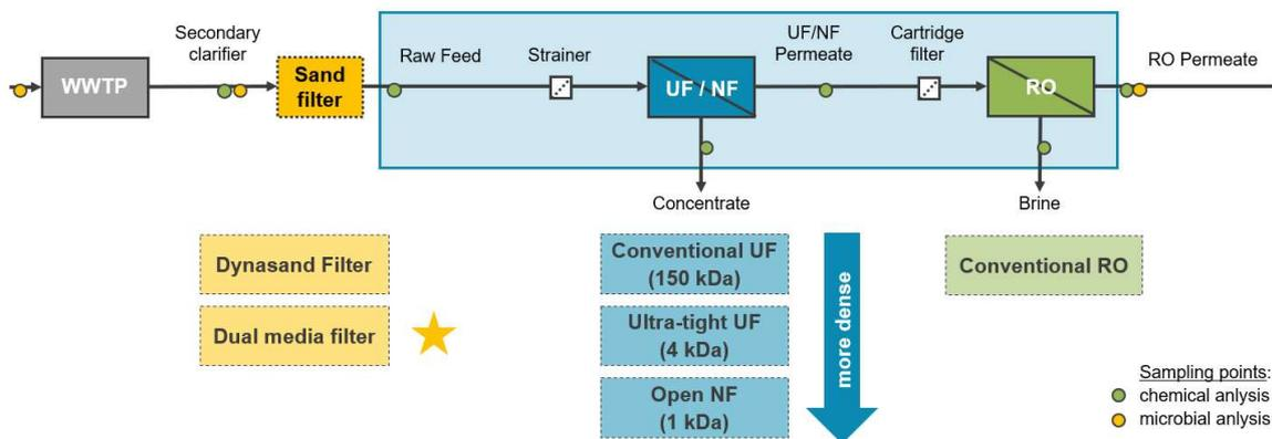
Figure 58. CS9: Pilot plant – flow scheme, tested pre-treatment and membranes and sampling points.
