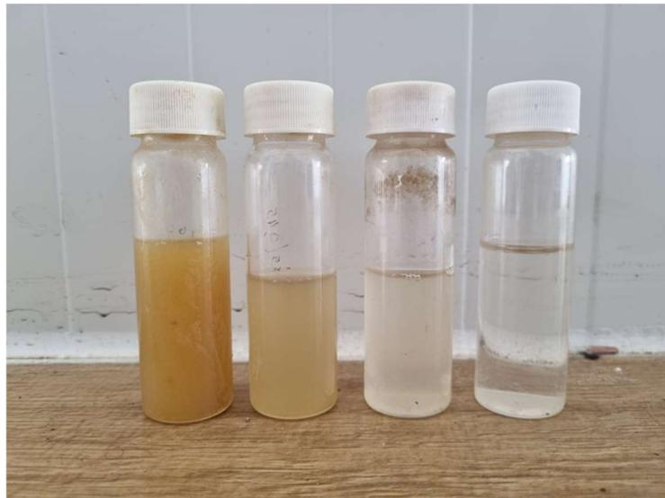
Figure 49. CS4: Inlet orange juice by product (left), intermediate semi-treated by-product and treated water (right).
