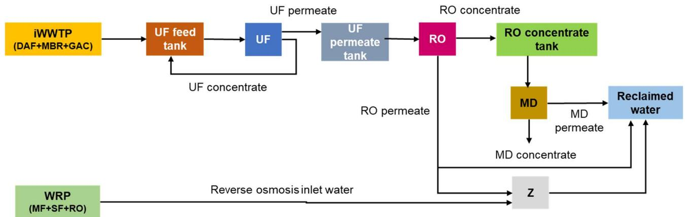
Figure 4. CS1: Pilot plant process scheme.
