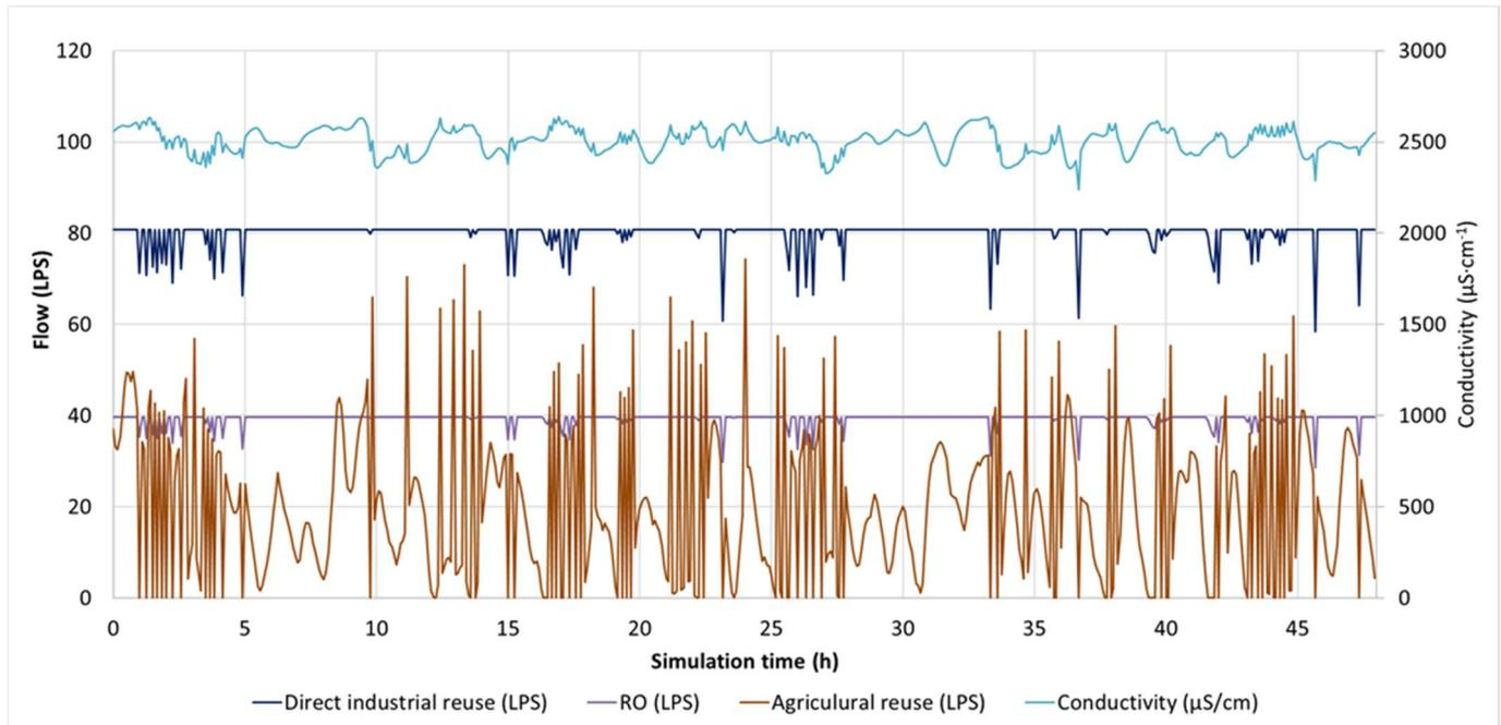
Figure 30. CS3: Evolution of the reclaimed water flows distributed by the matchmaking platform.
