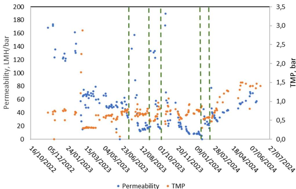
Figure 6. CS1: Ultrafiltration permeability and transmembrane pressure (max. 8 bar). Green dotted lines show CIP cleanings.
