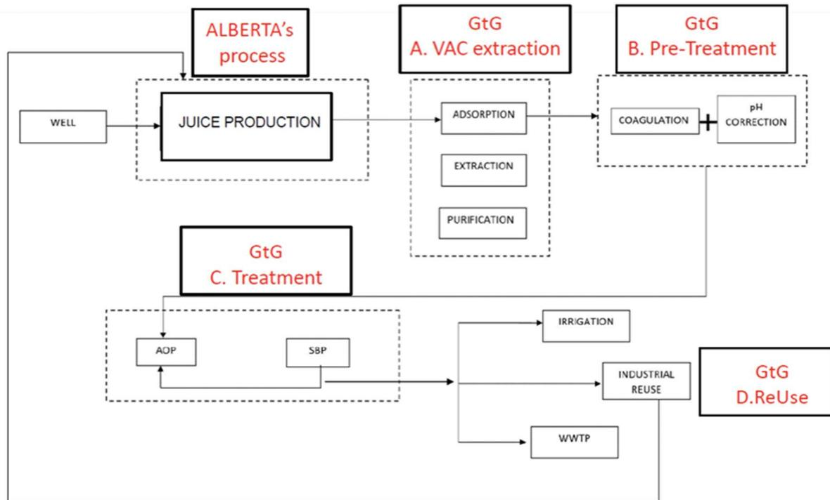
Figure 39. CS4: Layout of the pilot process deployed at Alberta S.A.
