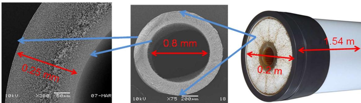
Figure 60. CS9: UF/NF membrane with microscopic details and dimensions of membrane fibres; left: fibre wall, middle: fibre, right: module head.
