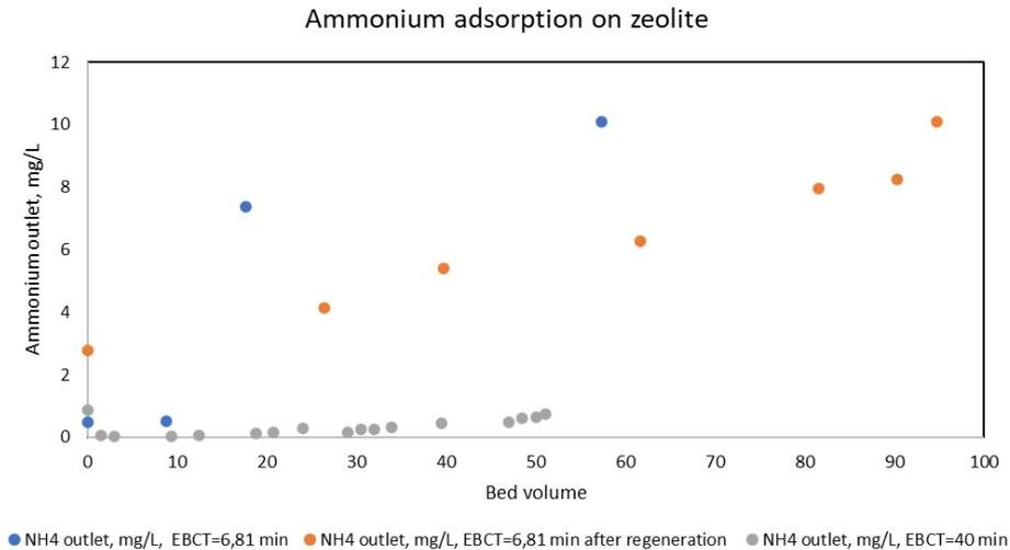
Figure 10. CS1: Ammonium adsorption on zeolites.
