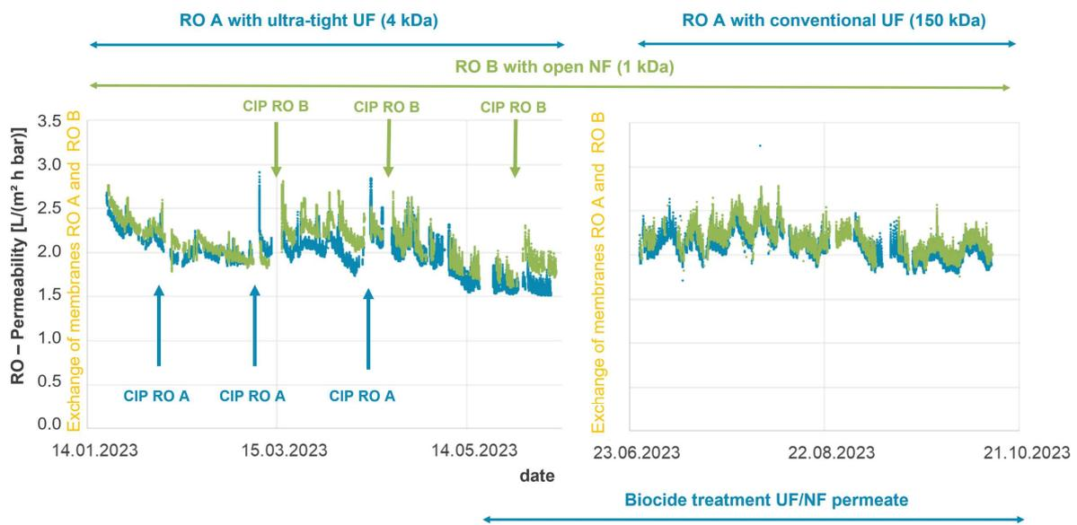
Figure 62. CS9: Permeability of RO with different pre-treatment membranes: (left): u-t UF and NF, (right): UF and NF with an intermittent biocide treatment of the RO feed (tanks and pipes).
