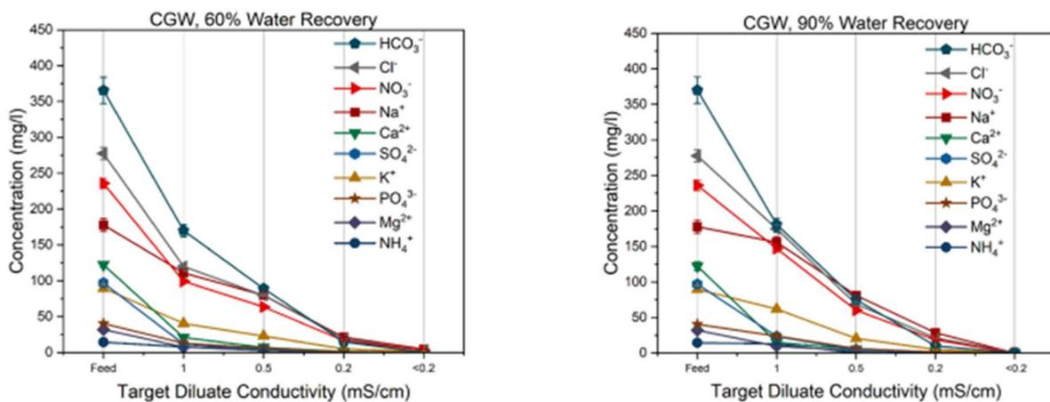
Figure 17. CS2: (C)ED ion transport and removal trends (60% and 90% water recovery, respectively).
