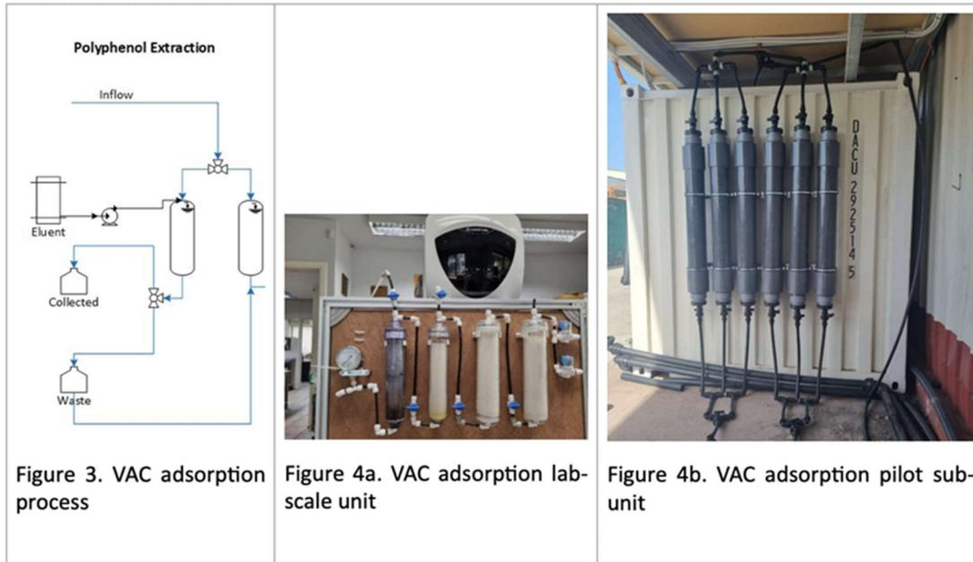
Figure 40. CS4: VAC adsorption process, VAC adsorption laboratory scale unit and VAC adsorption pilot sub-unit.
