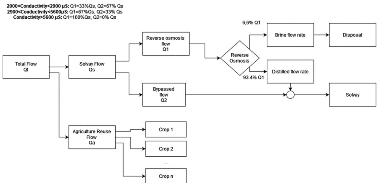
Figure 24. CS3: Logic of matchmaking platform.
