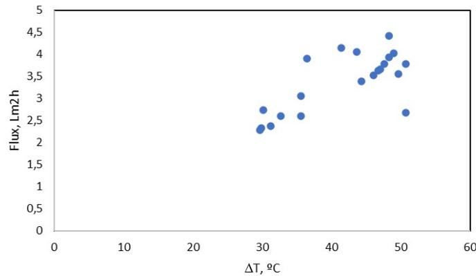
Figure 8. CS1: Membrane distillation permeability.
