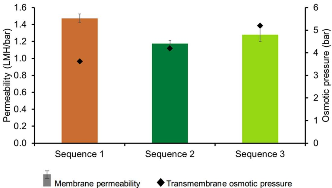
Figure 55. CS7: Osmotic pressure and permeability of the three sequences tested.
