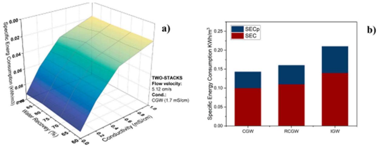
Figure 18. CS2: a) Specific energy consumption (SEC) in KWh/m<sup>3</sup> for desalinating greenhouse wastewater (CGW feed composition (EC 1.7 mS/cm)) using (C)ED. The colour gradient from light green to dark blue represents an increase in SEC corresponding to target conductivities (1 to <0.2 mS/cm), achieved over water recoveries of 60–90 %. b) Total energy consumption (SEC stack and SEC Pump) for all compositions and 90 % water recovery.
