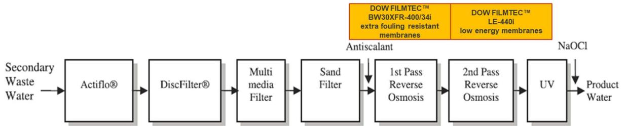
Figure 2. CS1: AITASA Water Reclamation Plant process scheme.
